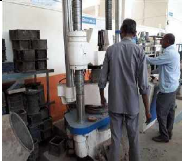
Concrete cube test using UTM
