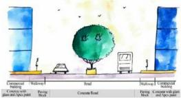
Figure 26: Schematic Section of Sinhgad road, pune
